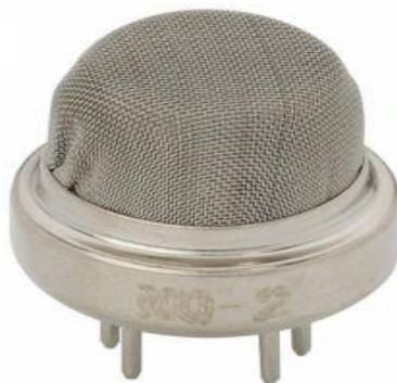
Fig 3 : Alcoholic sensor (MQ-2)
