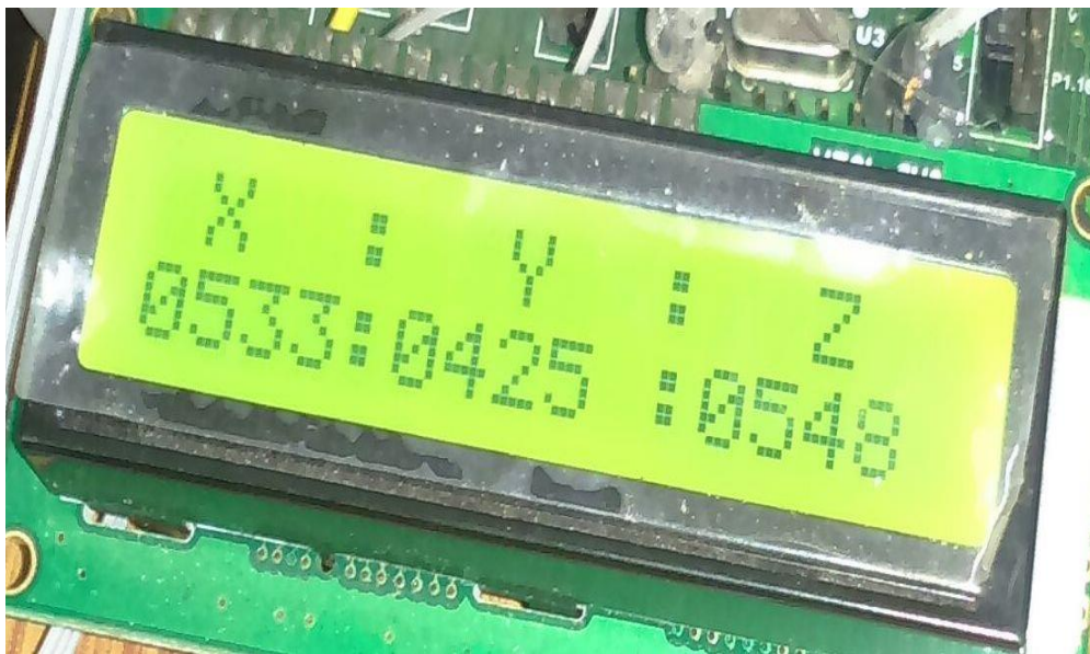
Fig 6: Readings of MEMs accelerometer
